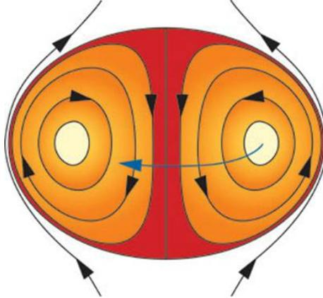
Figure 1: Simple axisymmetric spheromak (or FRC). Major and minor radii are both  $r$ . The height of the cylinder is  $2r$ ,
