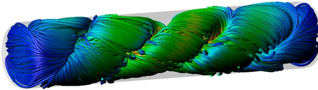
Figure 2: SSX Taylor state. Current flows in a twisted path, increasing the inductance and therefore lifetime for a given size.
