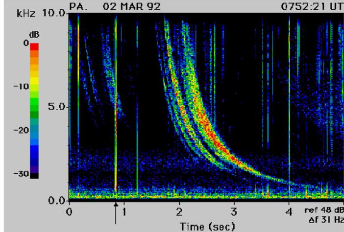
Figure 2: Whistler observation. Plot of the characteristic falling tone of a whistler wave recorded at Palmer Station, Antarctica. If played into a speaker, this would sound like a descending tone for about 2 seconds.
