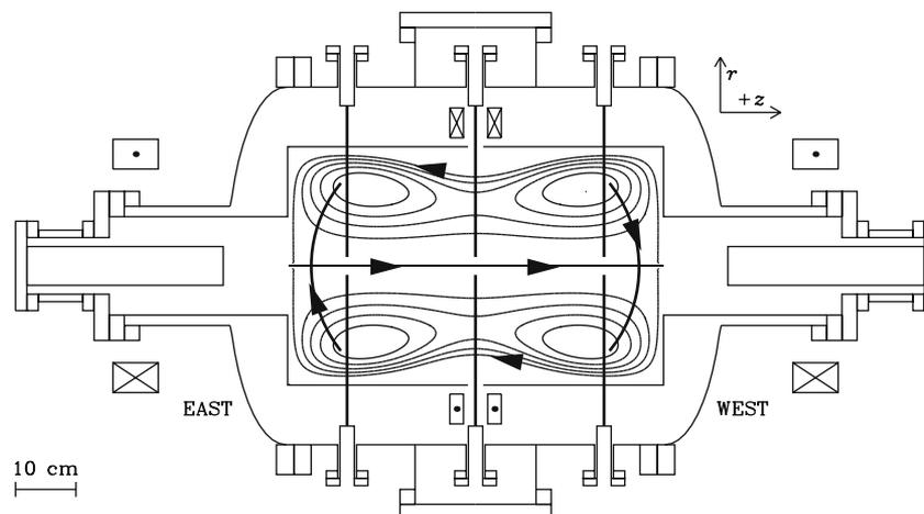
**Fig. 1.** The Swarthmore Spheromak Experiment (SSX) as configured for counter-helicity spheromak merging experiments, and flux surfaces for a Grad-Shafranov equilibrium for incomplete poloidal flux reconnection.
