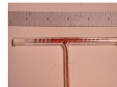
Figure 11. High-resolution magnetic probe. The cluster at the center of the T is actually 16 small coils placed directly next to each other in order to get a more specific reading of the magnetic fields at the reconnection region. The casing is quartz and the plugs on the ends of the T are boron nitride.
